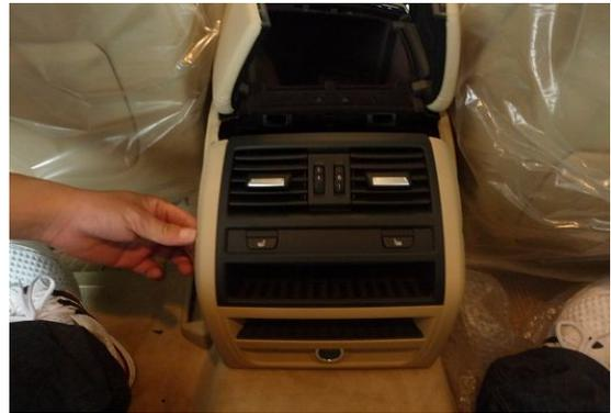
7) Remove rail box back tuyere cover, pull out cigarette lighter plug connection ACC and ground and AUX audio line
