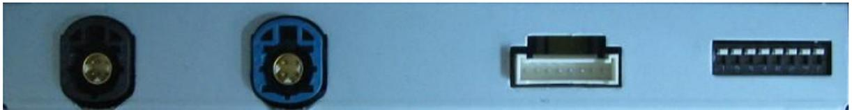
↑      LCD-OUT (data output)      LCD-IN (data input)      ↑      Slot of pallet      ↑      Function Setup
